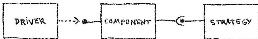
Figure 6.16: Component + Strategy as a component diagram (Image courtesy of Juan Manuel Garrido de Paz)
